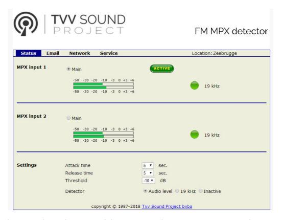
This page shows the status of the 2 connected sources: MPX input2 and MPX input2. . By way of the radio buttons (Main) can be selected which source is used as the main input, and be switched to the output provided that it has a signal. This will be indicated with the text ACTIVE. The meters show whether signal is present. On every input, there is also an indicator for 19kHz. If it is present, the indicator is green, and otherwise it is red.
