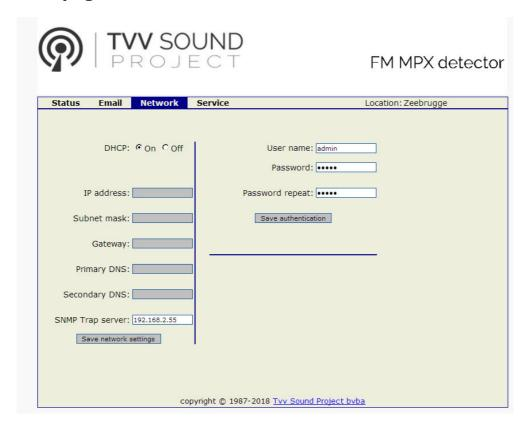
The 3<sup>rd</sup> page is for configuring the IP address and the password for logging into the web pages of the detector.
