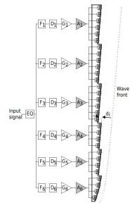
StepArray columns implement the DGRC line-array principle (Digital and Geometric Radiation control) which is a synthesis of geometric and electronic arrays patented by Active audio.
